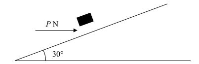
A parcel of weight 10 N lies on a rough plane inclined at an angle of  $30^{\circ}$  to the horizontal. A horizontal force of magnitude P newtons acts on the parcel, as shown in Figure 2. The parcel is in equilibrium and on the point of slipping up the plane. The normal reaction of the plane on the parcel is 18 N. The coefficient of friction between the parcel and the plane is  $\mu$ . Find
