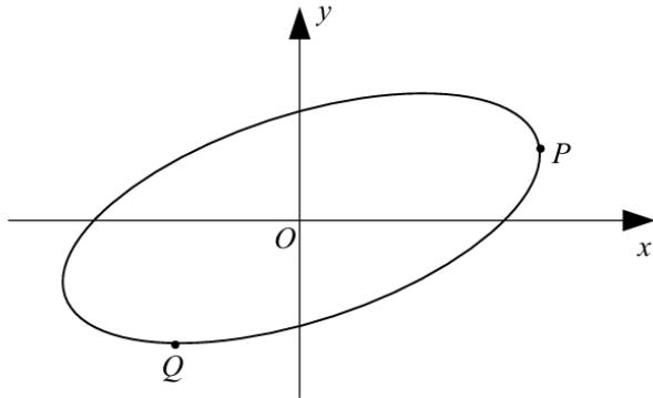
The diagram shows the curve with equation  $x^2 - 2xy + 4y^2 - 12 = 0$
