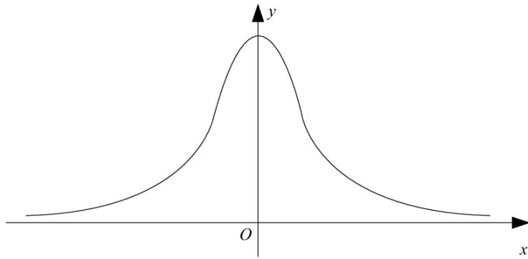
The diagram shows the curve with the equation  $y = \frac{1}{1+x^2}$
