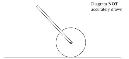
Trundle wheels are used to measure distances along the ground.
